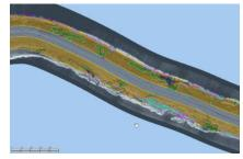
Figure 2: Example of the processed sidescan sonar imagery that has drawn polygons of different classes of substrate calculated using the SonarWiz Seabed Classification tool.
