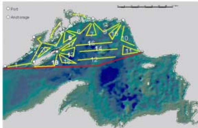
Figure 1. Proposed transect lines for hydroacoustic sampling to be performed in August of 2003. This design assumes a mean sampling speed of approximately 5 knots and 20 sample dates.
