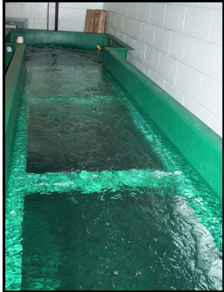
This test flume mimics a natural stream channel, allowing scientists to observe fish and sea lamprey swimming behavior, reactions to varying current eddies and velocities, and reactions to pheromones in the water.
